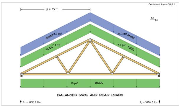
$$\begin{split} R_1 &= D + S = 2606.8 \text{ lbs} + 3189.8 \text{ lbs} \\ R_2 &= D + S = 2606.8 \text{ lbs} + 3189.8 \text{ lbs} \end{split}$$
