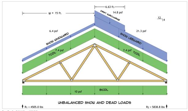
$R_1 = D + S = 2606.8 \text{ lbs} + 1898.2 \text{ lbs} \\ R_2 = D + S = 2606.8 \text{ lbs} + 3232.0 \text{ lbs}$
