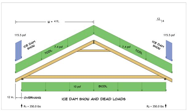
$$\begin{split} R_1 &= D + S = 119.0 \text{ lbs} + 231.0 \text{ lbs} \\ R_2 &= D + S = 119.0 \text{ lbs} + 231.0 \text{ lbs} \end{split}$$
