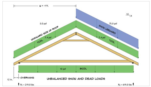
$R_1 = D + S = 119.0 \text{ lbs} + 100.0 \text{ lbs}$  $R_2 = D + S = 119.0 \text{ lbs} + 500.0 \text{ lbs}$
