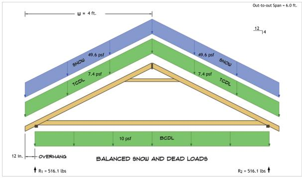
$R_1 = D + S = 119.0 \text{ lbs} + 397.1 \text{ lbs}$  $R_2 = D + S = 119.0 \text{ lbs} + 397.1 \text{ lbs}$
