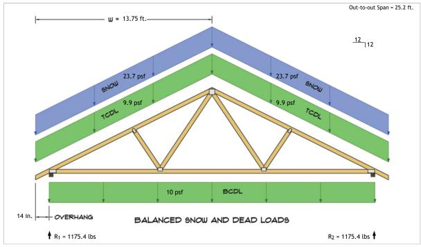
$R_1 = D + S = 523.9 \text{ lbs} + 651.5 \text{ lbs}$  $R_2 = D + S = 523.9 \text{ lbs} + 651.5 \text{ lbs}$
