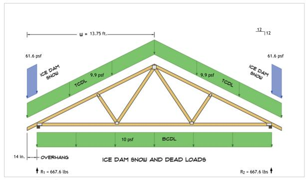
$R_1 = D + S = 523.9 \text{ lbs} + 143.7 \text{ lbs}$  $R_2 = D + S = 523.9 \text{ lbs} + 143.7 \text{ lbs}$
