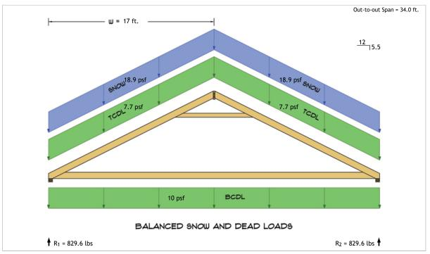
$R_1 = D + S = 401.2 \text{ lbs} + 428.4 \text{ lbs}$  $R_2 = D + S = 401.2 \text{ lbs} + 428.4 \text{ lbs}$
