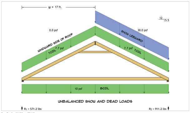
$R_1 = D + S = 401.2 \text{ lbs} + 170.0 \text{ lbs}$  $R_2 = D + S = 401.2 \text{ lbs} + 510.0 \text{ lbs}$
