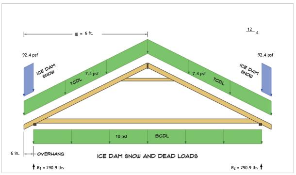
$$\begin{split} R_1 &= D + S = 198.5 \text{ lbs} + 92.4 \text{ lbs} \\ R_2 &= D + S = 198.5 \text{ lbs} + 92.4 \text{ lbs} \end{split}$$
