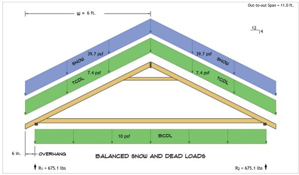
$R_1 = D + S = 198.5 \text{ lbs} + 476.5 \text{ lbs}$  $R_2 = D + S = 198.5 \text{ lbs} + 476.5 \text{ lbs}$
