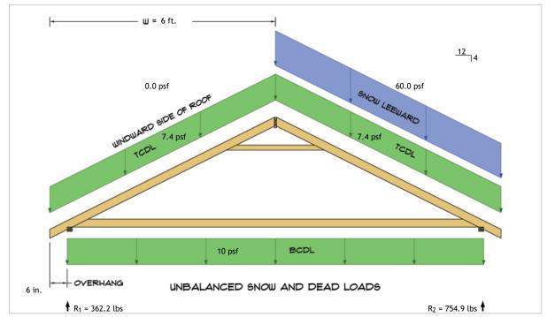
$R_1 = D + S = 198.5 \text{ lbs} + 163.6 \text{ lbs}$  $R_2 = D + S = 198.5 \text{ lbs} + 556.4 \text{ lbs}$
