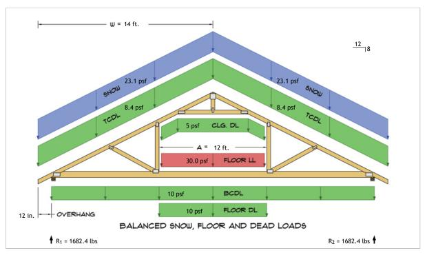
$$\begin{split} R_1 &= D + 0.75L + 0.75S = 675.6 \text{ lbs} + 360.0 \text{ lbs} + 646.8 \text{ lbs} \\ R_2 &= D + 0.75L + 0.75S = 675.6 \text{ lbs} + 360.0 \text{ lbs} + 646.8 \text{ lbs} \end{split}$$
