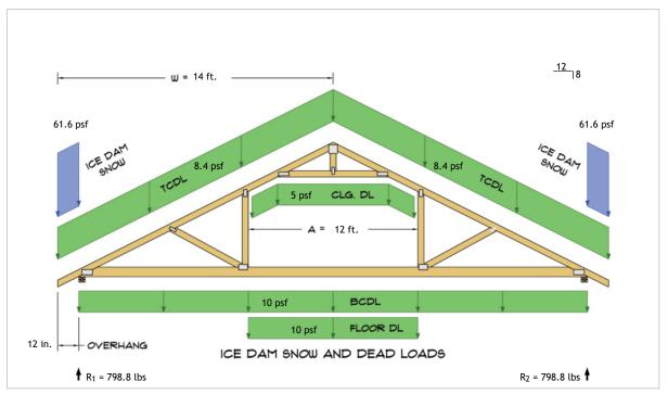
$R_1 = D + S = 675.6 \text{ lbs} + 123.2 \text{ lbs}$  $R_2 = D + S = 675.6 \text{ lbs} + 123.2 \text{ lbs}$
