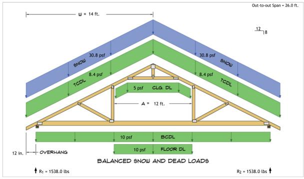
$R_1 = D + S = 675.6 \text{ lbs} + 862.4 \text{ lbs}$  $R_2 = D + S = 675.6 \text{ lbs} + 862.4 \text{ lbs}$
