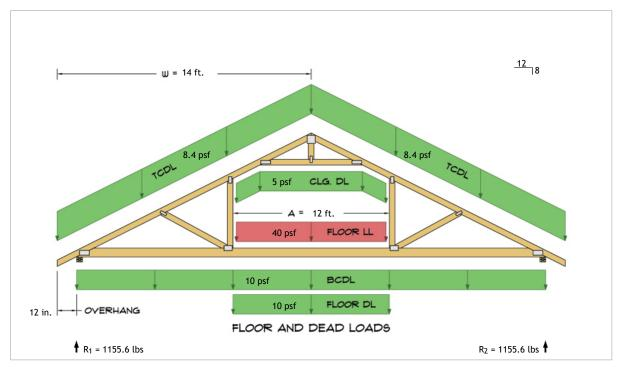
$R_1 = D + L = 675.6 \text{ lbs} + 480.0 \text{ lbs} \\ R_2 = D + L = 675.6 \text{ lbs} + 480.0 \text{ lbs}$
