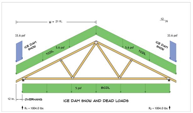
$$\begin{split} R_1 &= D + S = 869.6 \text{ lbs} + 134.4 \text{ lbs} \\ R_2 &= D + S = 869.6 \text{ lbs} + 134.4 \text{ lbs} \end{split}$$
