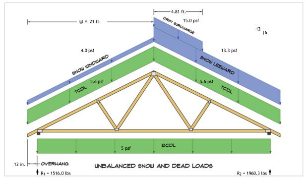
$R_1 = D + S = 869.6 \text{ lbs} + 646.4 \text{ lbs} \\ R_2 = D + S = 869.6 \text{ lbs} + 1090.7 \text{ lbs}$
