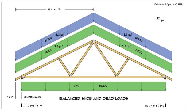
$\begin{aligned} R_1 &= D + S = 869.6 \text{ lbs} + 1114.3 \text{ lbs} \\ R_2 &= D + S = 869.6 \text{ lbs} + 1114.3 \text{ lbs} \end{aligned}$
