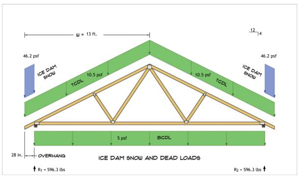
$$\begin{split} R_1 &= D + S = 380.7 \text{ lbs} + 215.6 \text{ lbs} \\ R_2 &= D + S = 380.7 \text{ lbs} + 215.6 \text{ lbs} \end{split}$$
