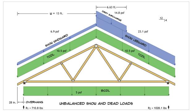
$R_1 = D + S = 380.7 \text{ lbs} + 330.1 \text{ lbs}$  $R_2 = D + S = 380.7 \text{ lbs} + 647.4 \text{ lbs}$
