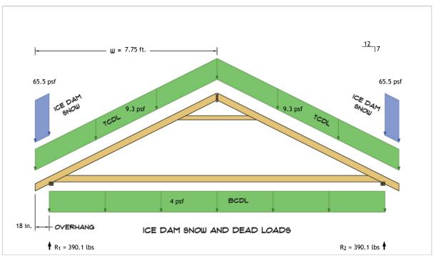
$$\begin{split} R_1 &= D + S = 193.6 \text{ lbs} + 196.6 \text{ lbs} \\ R_2 &= D + S = 193.6 \text{ lbs} + 196.6 \text{ lbs} \end{split}$$
