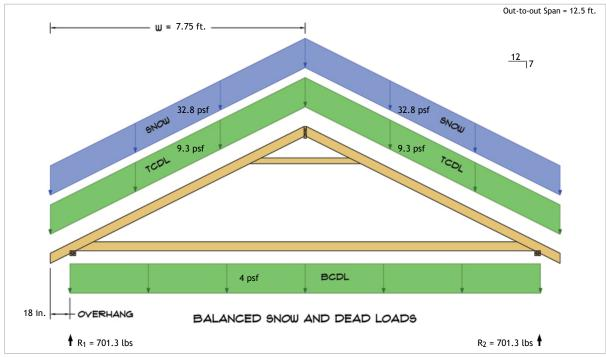
$R_1 = D + S = 193.6 \text{ lbs} + 507.8 \text{ lbs}$  $R_2 = D + S = 193.6 \text{ lbs} + 507.8 \text{ lbs}$
