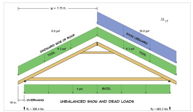
$R_1 = D + S = 193.6 \text{ lbs} + 114.9 \text{ lbs}$  $R_2 = D + S = 193.6 \text{ lbs} + 489.6 \text{ lbs}$
