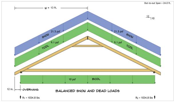
$R_1 = D + S = 476.9 \text{ lbs} + 557.9 \text{ lbs}$  $R_2 = D + S = 476.9 \text{ lbs} + 557.9 \text{ lbs}$
