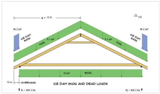
$R_1 = D + S = 476.9 \text{ lbs} + 92.4 \text{ lbs} \\ R_2 = D + S = 476.9 \text{ lbs} + 92.4 \text{ lbs}$
