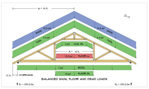
$$\begin{split} R_1 &= D + 0.75L + 0.75S = 513.3 \text{ lbs} + 150.0 \text{ lbs} + 729.7 \text{ lbs} \\ R_2 &= D + 0.75L + 0.75S = 513.3 \text{ lbs} + 150.0 \text{ lbs} + 729.7 \text{ lbs} \end{split}$$
