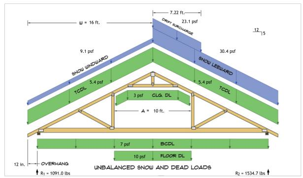
$R_1 = D + S = 513.3 \text{ lbs} + 577.7 \text{ lbs}$  $R_2 = D + S = 513.3 \text{ lbs} + 1021.3 \text{ lbs}$
