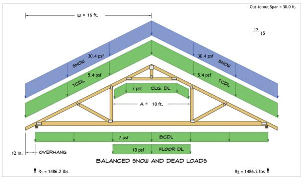
$$\begin{split} R_1 &= D + S = 513.3 \text{ lbs} + 972.9 \text{ lbs} \\ R_2 &= D + S = 513.3 \text{ lbs} + 972.9 \text{ lbs} \end{split}$$
