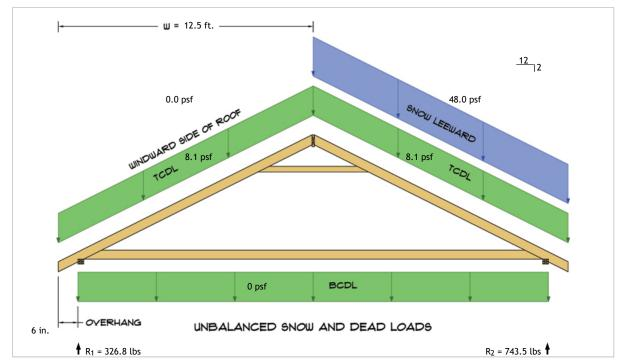
$R_1 = D + S = 135.2 \text{ lbs} + 191.7 \text{ lbs}$  $R_2 = D + S = 135.2 \text{ lbs} + 608.3 \text{ lbs}$
