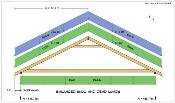
$R_1 = D + S = 135.2 \text{ lbs} + 521.6 \text{ lbs}$  $R_2 = D + S = 135.2 \text{ lbs} + 521.6 \text{ lbs}$
