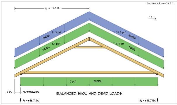
$R_1 = D + S = 135.2 \text{ lbs} + 521.6 \text{ lbs}$  $R_2 = D + S = 135.2 \text{ lbs} + 521.6 \text{ lbs}$
