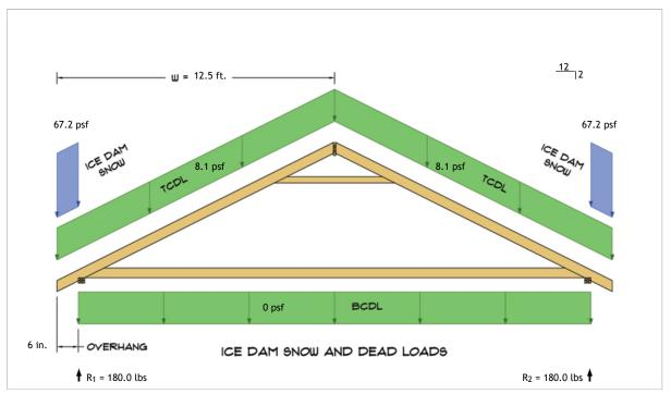
$$\begin{split} R_1 &= D + S = 135.2 \text{ lbs} + 44.8 \text{ lbs} \\ R_2 &= D + S = 135.2 \text{ lbs} + 44.8 \text{ lbs} \end{split}$$
