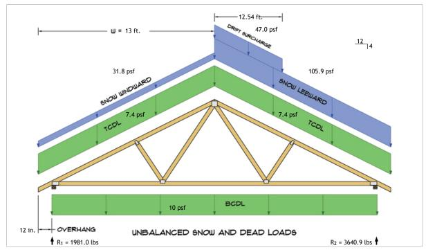
$R_1 = D + S = 431.8 \text{ lbs} + 1549.1 \text{ lbs}$  $R_2 = D + S = 431.8 \text{ lbs} + 3209.0 \text{ lbs}$
