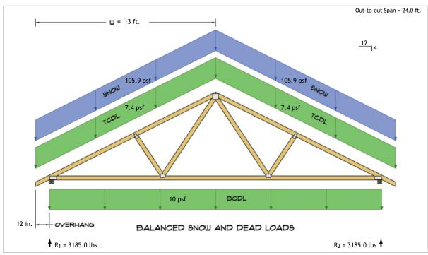
$\begin{aligned} R_1 &= D + S = 431.8 \text{ lbs} + 2753.2 \text{ lbs} \\ R_2 &= D + S = 431.8 \text{ lbs} + 2753.2 \text{ lbs} \end{aligned}$
