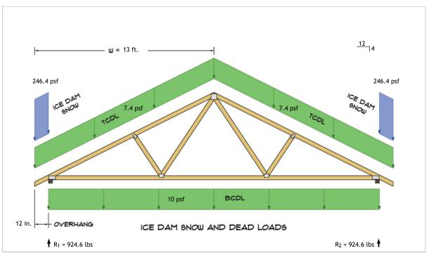
$R_1 = D + S = 431.8 \text{ lbs} + 492.8 \text{ lbs}$  $R_2 = D + S = 431.8 \text{ lbs} + 492.8 \text{ lbs}$
