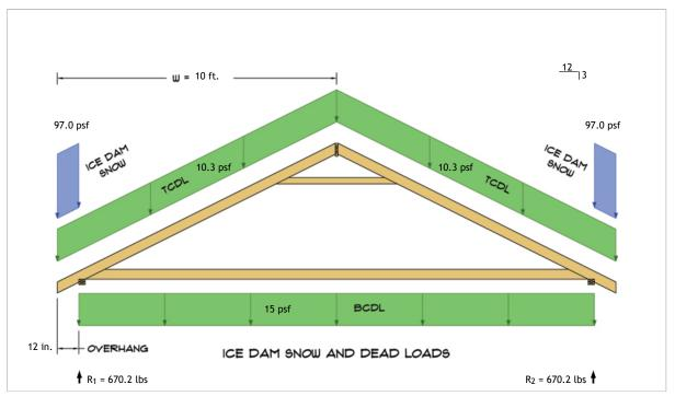
$$\begin{split} R_1 &= D + S = 476.2 \text{ lbs} + 194.0 \text{ lbs} \\ R_2 &= D + S = 476.2 \text{ lbs} + 194.0 \text{ lbs} \end{split}$$
