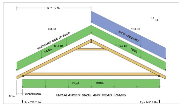
$R_1 = D + S = 476.2 \text{ lbs} + 280.0 \text{ lbs}$  $R_2 = D + S = 476.2 \text{ lbs} + 980.0 \text{ lbs}$
