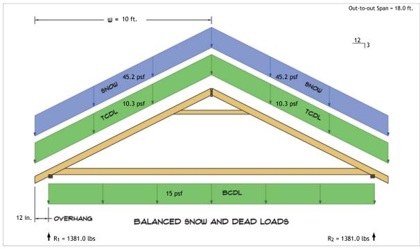
$R_1 = D + S = 476.2 \text{ lbs} + 904.9 \text{ lbs}$  $R_2 = D + S = 476.2 \text{ lbs} + 904.9 \text{ lbs}$
