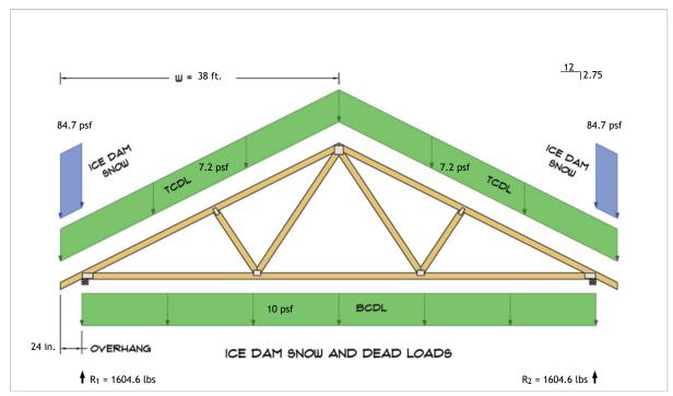
$$\begin{split} R_1 &= D + S = 1265.8 \text{ lbs} + 338.8 \text{ lbs} \\ R_2 &= D + S = 1265.8 \text{ lbs} + 338.8 \text{ lbs} \end{split}$$
