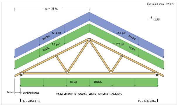
$$\begin{split} R_1 &= D + S = 1265.8 \text{ lbs} + 3218.6 \text{ lbs} \\ R_2 &= D + S = 1265.8 \text{ lbs} + 3218.6 \text{ lbs} \end{split}$$
