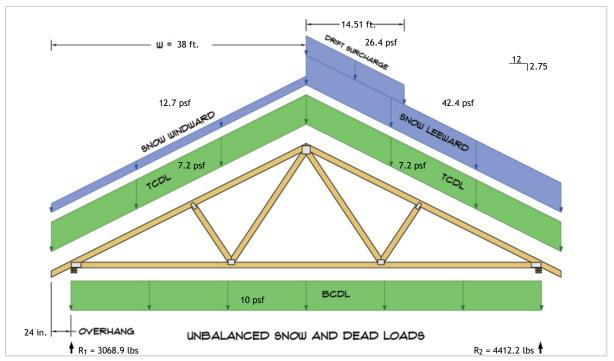
$R_1 = D + S = 1265.8 \text{ lbs} + 1803.1 \text{ lbs}$  $R_2 = D + S = 1265.8 \text{ lbs} + 3146.4 \text{ lbs}$
