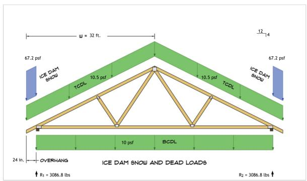
$R_1 = D + S = 2549.2 \text{ lbs} + 537.6 \text{ lbs}$  $R_2 = D + S = 2549.2 \text{ lbs} + 537.6 \text{ lbs}$
