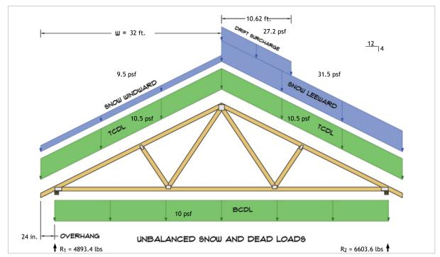
$R_1 = D + S = 2549.2 \text{ lbs} + 2344.2 \text{ lbs}$  $R_2 = D + S = 2549.2 \text{ lbs} + 4054.4 \text{ lbs}$
