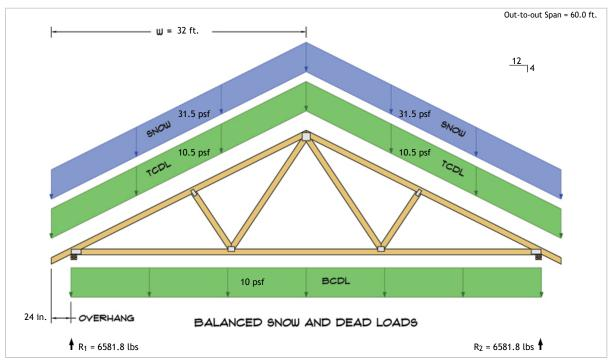
$$\begin{split} R_1 &= D + S = 2549.2 \text{ lbs} + 4032.6 \text{ lbs} \\ R_2 &= D + S = 2549.2 \text{ lbs} + 4032.6 \text{ lbs} \end{split}$$
