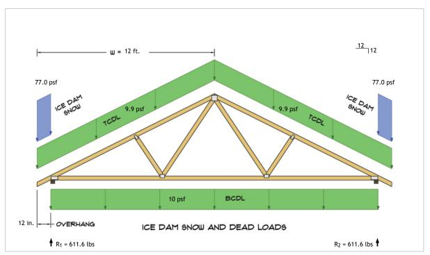
$R_1 = D + S = 457.6 \text{ lbs} + 154.0 \text{ lbs}$  $R_2 = D + S = 457.6 \text{ lbs} + 154.0 \text{ lbs}$
