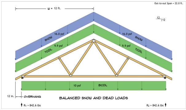
$R_1 = D + S = 457.6 \text{ lbs} + 385.0 \text{ lbs}$  $R_2 = D + S = 457.6 \text{ lbs} + 385.0 \text{ lbs}$
