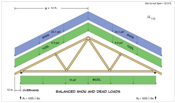
$R_1 = D + S = 457.6 \text{ lbs} + 577.5 \text{ lbs}$  $R_2 = D + S = 457.6 \text{ lbs} + 577.5 \text{ lbs}$
