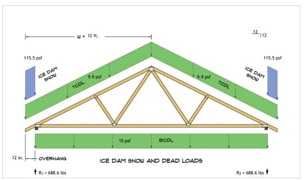
$R_1 = D + S = 457.6 \text{ lbs} + 231.0 \text{ lbs}$  $R_2 = D + S = 457.6 \text{ lbs} + 231.0 \text{ lbs}$
