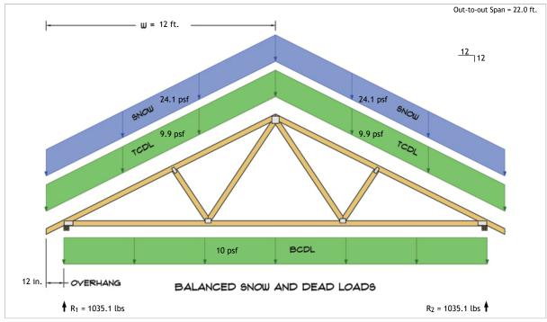
$R_1 = D + S = 457.6 \text{ lbs} + 577.5 \text{ lbs}$  $R_2 = D + S = 457.6 \text{ lbs} + 577.5 \text{ lbs}$
