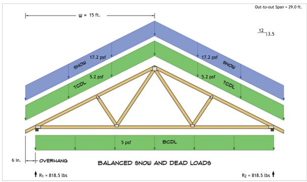
$$\begin{split} R_1 &= D + S = 301.3 \text{ lbs} + 517.2 \text{ lbs} \\ R_2 &= D + S = 301.3 \text{ lbs} + 517.2 \text{ lbs} \end{split}$$
