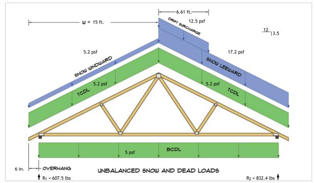
$R_1 = D + S = 301.3 \text{ lbs} + 306.2 \text{ lbs}$  $R_2 = D + S = 301.3 \text{ lbs} + 531.1 \text{ lbs}$
