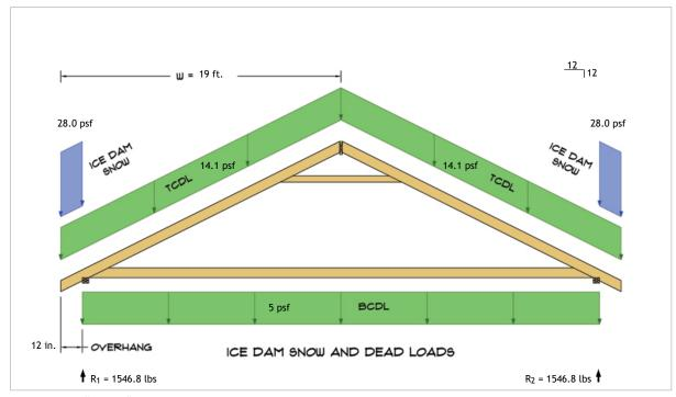
$R_1 = D + S = 1434.8 \text{ lbs} + 112.0 \text{ lbs}$  $R_2 = D + S = 1434.8 \text{ lbs} + 112.0 \text{ lbs}$
