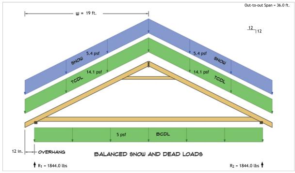
$R_1 = D + S = 1434.8 \text{ lbs} + 409.2 \text{ lbs}$  $R_2 = D + S = 1434.8 \text{ lbs} + 409.2 \text{ lbs}$
