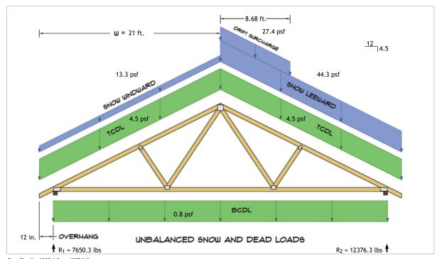
$R_1 = D + S = 1322.4 \text{ lbs} + 6327.9 \text{ lbs}$  $R_2 = D + S = 1322.4 \text{ lbs} + 11054.0 \text{ lbs}$
