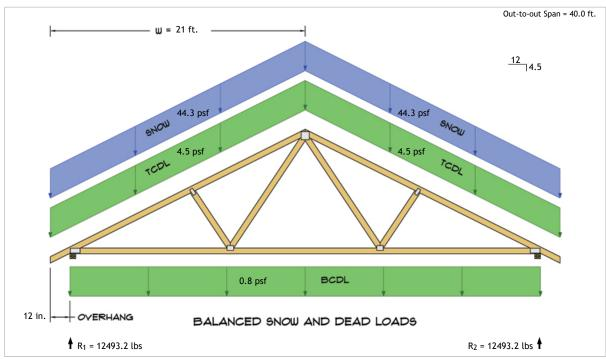
$$\begin{split} R_1 &= D + S = 1322.4 \text{ lbs} + 11170.8 \text{ lbs} \\ R_2 &= D + S = 1322.4 \text{ lbs} + 11170.8 \text{ lbs} \end{split}$$
