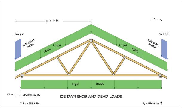
$$\begin{split} R_1 &= D + S = 464.2 \text{ lbs} + 92.4 \text{ lbs} \\ R_2 &= D + S = 464.2 \text{ lbs} + 92.4 \text{ lbs} \end{split}$$
