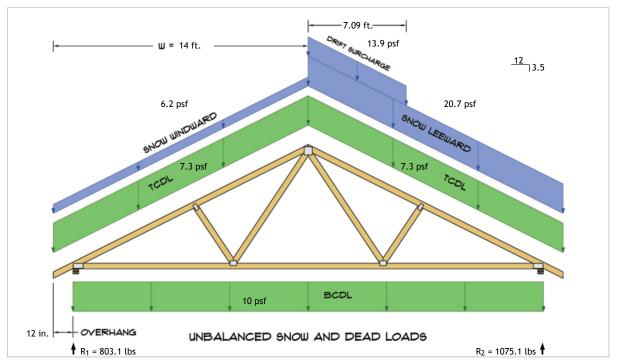
$R_1 = D + S = 464.2 \text{ lbs} + 338.9 \text{ lbs}$  $R_2 = D + S = 464.2 \text{ lbs} + 610.9 \text{ lbs}$
