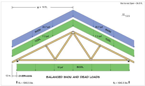
$$\begin{split} R_1 &= D + S = 464.2 \text{ lbs} + 579.3 \text{ lbs} \\ R_2 &= D + S = 464.2 \text{ lbs} + 579.3 \text{ lbs} \end{split}$$
