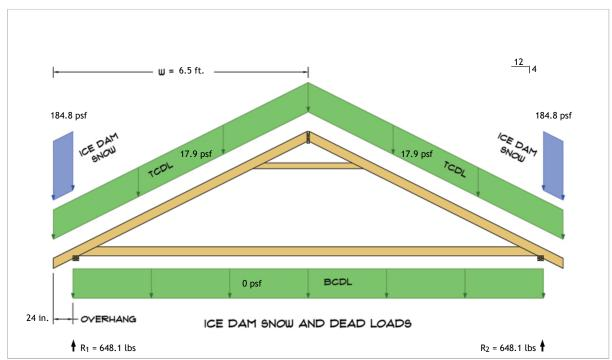
$R_1 = D + S = 155.3 \text{ lbs} + 492.8 \text{ lbs}$  $R_2 = D + S = 155.3 \text{ lbs} + 492.8 \text{ lbs}$
