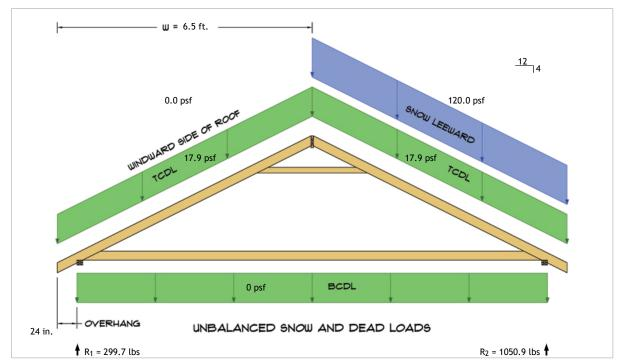
$R_1 = D + S = 155.3 \text{ lbs} + 144.4 \text{ lbs}$  $R_2 = D + S = 155.3 \text{ lbs} + 895.6 \text{ lbs}$
