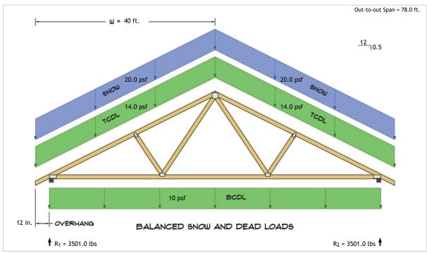
$$\begin{split} R_1 &= D + S = 1901.0 \text{ lbs} + 1600.0 \text{ lbs} \\ R_2 &= D + S = 1901.0 \text{ lbs} + 1600.0 \text{ lbs} \end{split}$$
