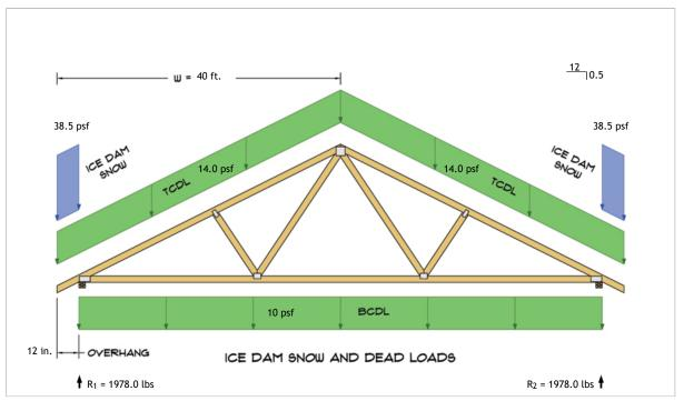
$$\begin{split} R_1 &= D + S = 1901.0 \text{ lbs} + 77.0 \text{ lbs} \\ R_2 &= D + S = 1901.0 \text{ lbs} + 77.0 \text{ lbs} \end{split}$$
