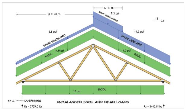
$R_1 = D + S = 1901.0 \text{ lbs} + 854.0 \text{ lbs}$  $R_2 = D + S = 1901.0 \text{ lbs} + 1544.9 \text{ lbs}$
