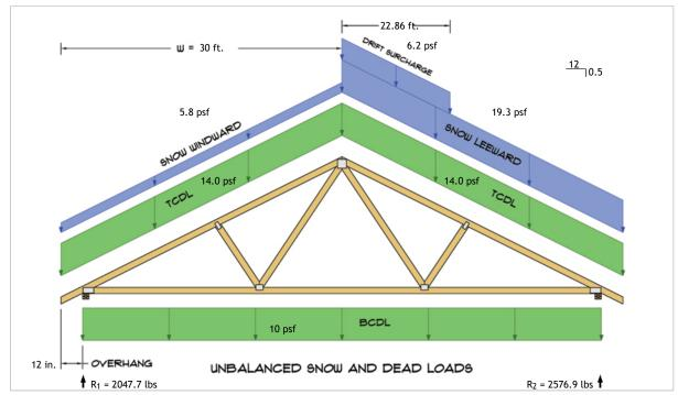
$R_1 = D + S = 1420.7 \text{ lbs} + 627.0 \text{ lbs}$  $R_2 = D + S = 1420.7 \text{ lbs} + 1156.2 \text{ lbs}$
