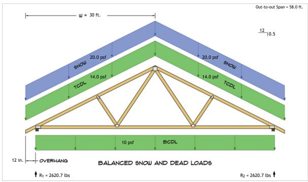
$$\begin{split} R_1 &= D + S = 1420.7 \text{ lbs} + 1200.0 \text{ lbs} \\ R_2 &= D + S = 1420.7 \text{ lbs} + 1200.0 \text{ lbs} \end{split}$$
