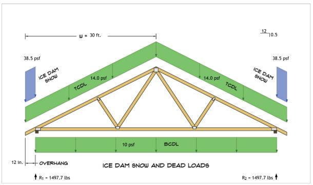
$$\begin{split} R_1 &= D + S = 1420.7 \text{ lbs} + 77.0 \text{ lbs} \\ R_2 &= D + S = 1420.7 \text{ lbs} + 77.0 \text{ lbs} \end{split}$$
