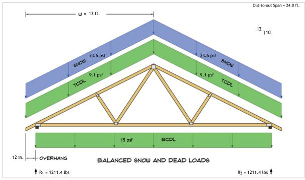
$R_1 = D + S = 596.9 \text{ lbs} + 614.5 \text{ lbs}$  $R_2 = D + S = 596.9 \text{ lbs} + 614.5 \text{ lbs}$
