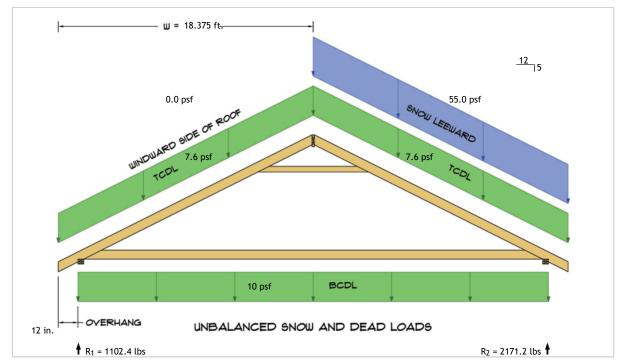
$R_1 = D + S = 626.2 \text{ lbs} + 476.2 \text{ lbs}$  $R_2 = D + S = 626.2 \text{ lbs} + 1545.0 \text{ lbs}$
