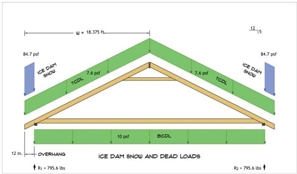
$$\begin{split} R_1 &= D + S = 626.2 \text{ lbs} + 169.4 \text{ lbs} \\ R_2 &= D + S = 626.2 \text{ lbs} + 169.4 \text{ lbs} \end{split}$$
