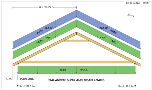
$R_1 = D + S = 626.2 \text{ lbs} + 1556.4 \text{ lbs}$  $R_2 = D + S = 626.2 \text{ lbs} + 1556.4 \text{ lbs}$
