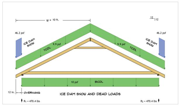
$R_1 = D + S = 378.0 \text{ lbs} + 92.4 \text{ lbs} \\ R_2 = D + S = 378.0 \text{ lbs} + 92.4 \text{ lbs}$
