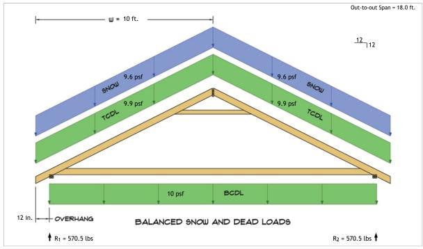
$R_1 = D + S = 378.0 \text{ lbs} + 192.5 \text{ lbs}$  $R_2 = D + S = 378.0 \text{ lbs} + 192.5 \text{ lbs}$
