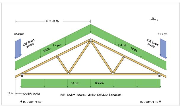
$R_1 = D + S = 1697.9 \text{ lbs} + 336.0 \text{ lbs}$  $R_2 = D + S = 1697.9 \text{ lbs} + 336.0 \text{ lbs}$
