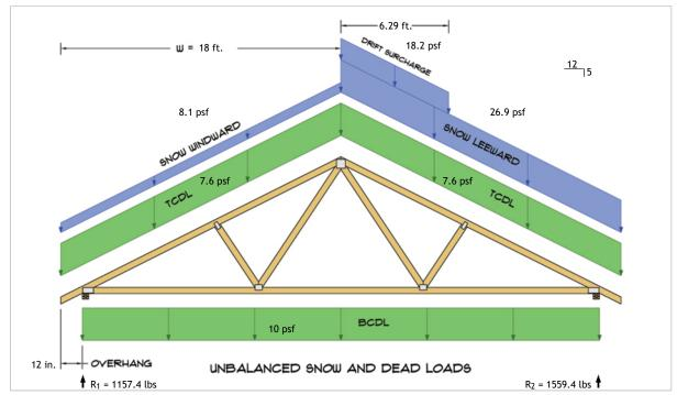
$R_1 = D + S = 613.0 \text{ lbs} + 544.4 \text{ lbs}$  $R_2 = D + S = 613.0 \text{ lbs} + 946.4 \text{ lbs}$
