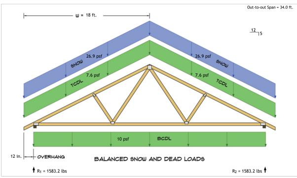
$$\begin{split} R_1 &= D + S = 613.0 \text{ lbs} + 970.2 \text{ lbs} \\ R_2 &= D + S = 613.0 \text{ lbs} + 970.2 \text{ lbs} \end{split}$$
