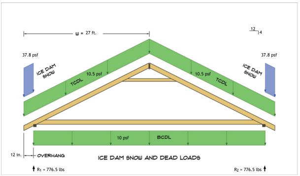
$$\begin{split} R_1 &= D + S = 726.1 \text{ lbs} + 50.4 \text{ lbs} \\ R_2 &= D + S = 726.1 \text{ lbs} + 50.4 \text{ lbs} \end{split}$$
