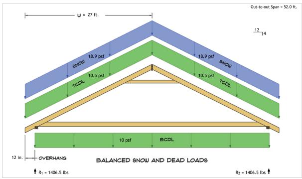
$$\begin{split} R_1 &= D + S = 726.1 \text{ lbs} + 680.4 \text{ lbs} \\ R_2 &= D + S = 726.1 \text{ lbs} + 680.4 \text{ lbs} \end{split}$$
