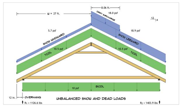
$R_1 = D + S = 726.1 \text{ lbs} + 400.4 \text{ lbs}$  $R_2 = D + S = 726.1 \text{ lbs} + 677.7 \text{ lbs}$
