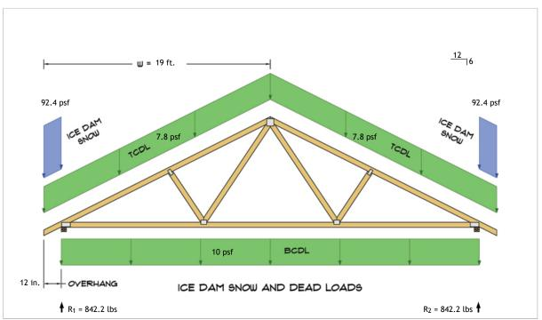
$R_1 = D + S = 657.4 \text{ lbs} + 184.8 \text{ lbs}$  $R_2 = D + S = 657.4 \text{ lbs} + 184.8 \text{ lbs}$
