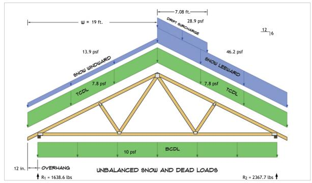
$R_1 = D + S = 657.4 \text{ lbs} + 981.2 \text{ lbs}$  $R_2 = D + S = 657.4 \text{ lbs} + 1710.3 \text{ lbs}$
