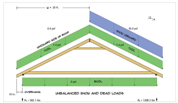
$R_1 = D + S = 295.1 \text{ lbs} + 287.0 \text{ lbs}$  $R_2 = D + S = 295.1 \text{ lbs} + 913.0 \text{ lbs}$
