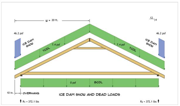
$\begin{aligned} R_1 &= D + S = 295.1 \text{ lbs} + 77.0 \text{ lbs} \\ R_2 &= D + S = 295.1 \text{ lbs} + 77.0 \text{ lbs} \end{aligned}$
