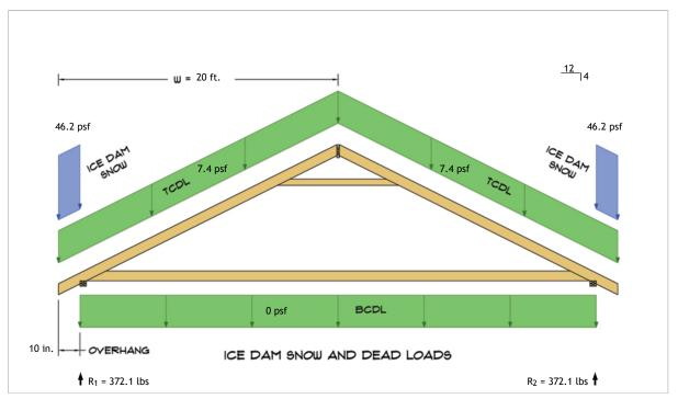
$$\begin{split} R_1 &= D + S = 295.1 \text{ lbs} + 77.0 \text{ lbs} \\ R_2 &= D + S = 295.1 \text{ lbs} + 77.0 \text{ lbs} \end{split}$$
