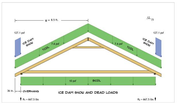
$$\begin{split} R_1 &= D + S = 159.3 \text{ lbs} + 508.2 \text{ lbs} \\ R_2 &= D + S = 159.3 \text{ lbs} + 508.2 \text{ lbs} \end{split}$$
