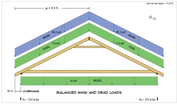
$R_1 = D + S = 159.3 \text{ lbs} + 568.5 \text{ lbs}$  $R_2 = D + S = 159.3 \text{ lbs} + 568.5 \text{ lbs}$
