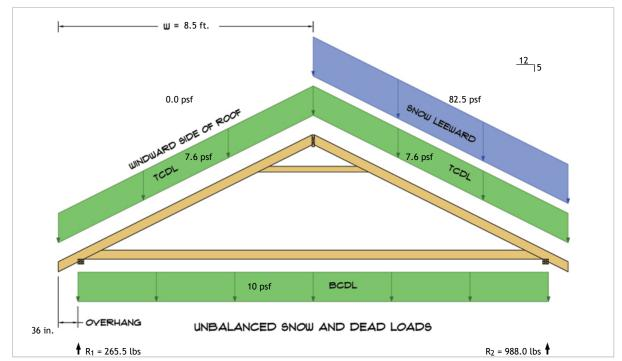
$R_1 = D + S = 159.3 \text{ lbs} + 106.3 \text{ lbs}$  $R_2 = D + S = 159.3 \text{ lbs} + 828.8 \text{ lbs}$
