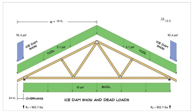
$$\begin{split} R_1 &= D + S = 534.1 \text{ lbs} + 369.6 \text{ lbs} \\ R_2 &= D + S = 534.1 \text{ lbs} + 369.6 \text{ lbs} \end{split}$$
