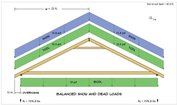
$\begin{aligned} R_1 &= D + S = 883.8 \text{ lbs} + 693.0 \text{ lbs} \\ R_2 &= D + S = 883.8 \text{ lbs} + 693.0 \text{ lbs} \end{aligned}$
