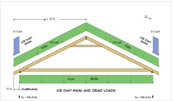
$R_1 = D + S = 883.8 \text{ lbs} + 63.0 \text{ lbs}$  $R_2 = D + S = 883.8 \text{ lbs} + 63.0 \text{ lbs}$
