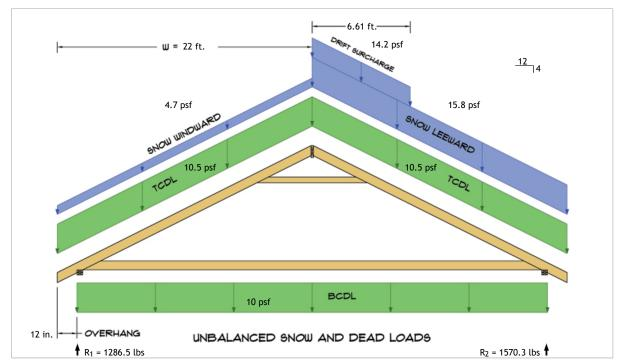
$$\begin{split} R_1 &= D + S = 883.8 \text{ lbs} + 402.7 \text{ lbs} \\ R_2 &= D + S = 883.8 \text{ lbs} + 686.5 \text{ lbs} \end{split}$$
