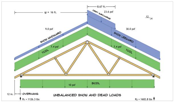
$R_1 = D + S = 536.1 \text{ lbs} + 590.2 \text{ lbs}$  $R_2 = D + S = 536.1 \text{ lbs} + 1066.7 \text{ lbs}$
