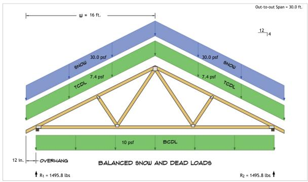
$$\begin{split} R_1 &= D + S = 536.1 \text{ lbs} + 959.7 \text{ lbs} \\ R_2 &= D + S = 536.1 \text{ lbs} + 959.7 \text{ lbs} \end{split}$$
