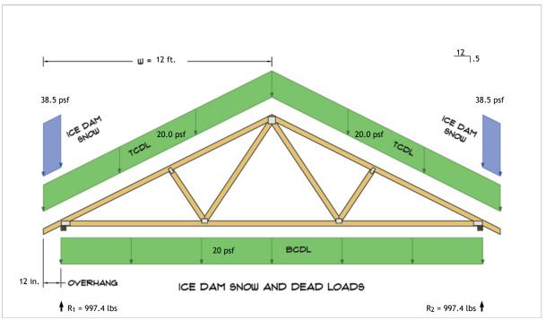
$R_1 = D + S = 920.4 \text{ lbs} + 77.0 \text{ lbs}$  $R_2 = D + S = 920.4 \text{ lbs} + 77.0 \text{ lbs}$
