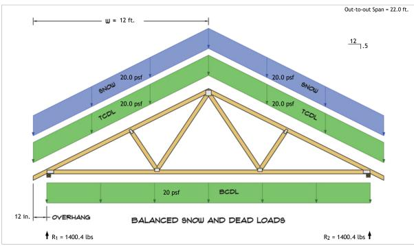
$$\begin{split} R_1 &= D + S = 920.4 \text{ lbs} + 480.0 \text{ lbs} \\ R_2 &= D + S = 920.4 \text{ lbs} + 480.0 \text{ lbs} \end{split}$$
