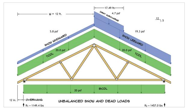
$R_1 = D + S = 920.4 \text{ lbs} + 229.0 \text{ lbs}$  $R_2 = D + S = 920.4 \text{ lbs} + 536.5 \text{ lbs}$
