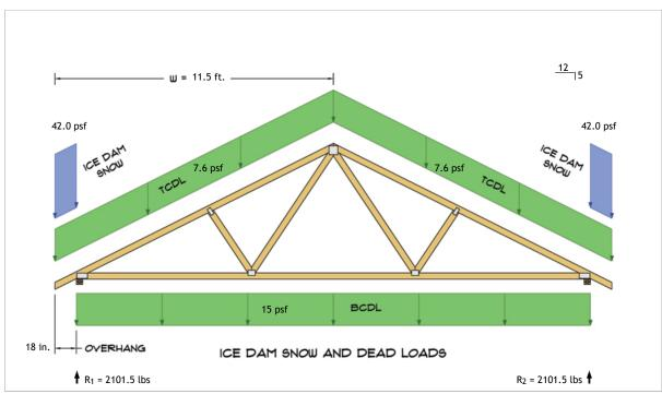
$R_1 = D + S = 1660.5 \text{ lbs} + 441.0 \text{ lbs}$  $R_2 = D + S = 1660.5 \text{ lbs} + 441.0 \text{ lbs}$
