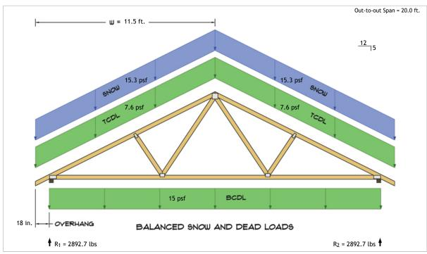
$$\begin{split} R_1 &= D + S = 1660.5 \text{ lbs} + 1232.2 \text{ lbs} \\ R_2 &= D + S = 1660.5 \text{ lbs} + 1232.2 \text{ lbs} \end{split}$$
