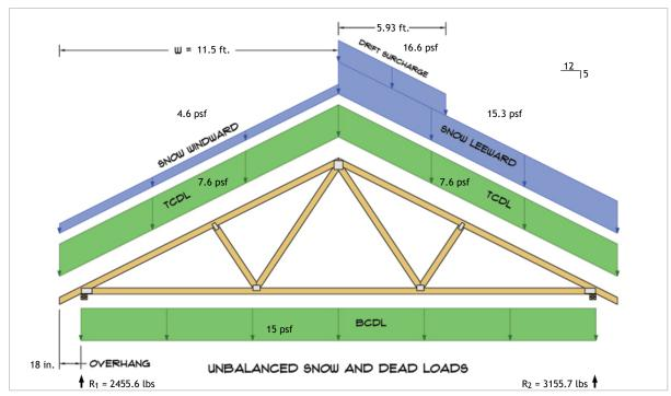
$R_1 = D + S = 1660.5 \text{ lbs} + 795.1 \text{ lbs}$  $R_2 = D + S = 1660.5 \text{ lbs} + 1495.2 \text{ lbs}$
