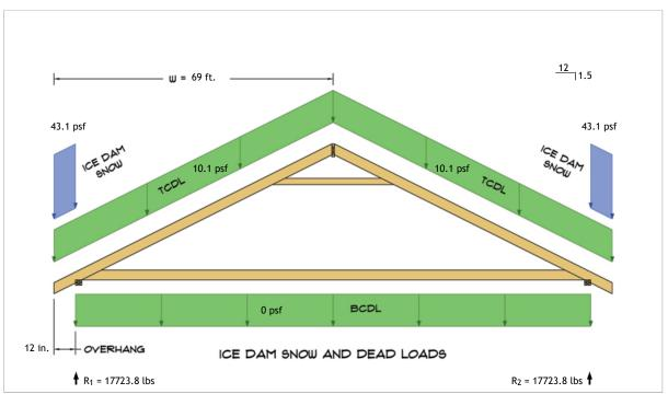
$R_1 = D + S = 16688.9 \text{ lbs} + 1034.9 \text{ lbs}$  $R_2 = D + S = 16688.9 \text{ lbs} + 1034.9 \text{ lbs}$
