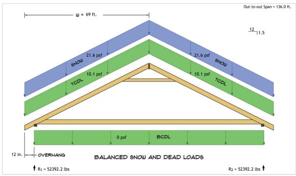
$$\begin{split} R_1 &= D + S = 16688.9 \text{ lbs} + 35703.4 \text{ lbs} \\ R_2 &= D + S = 16688.9 \text{ lbs} + 35703.4 \text{ lbs} \end{split}$$
