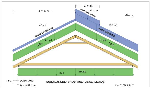
$R_1 = D + S = 16688.9 \text{ lbs} + 21503.7 \text{ lbs}$  $R_2 = D + S = 16688.9 \text{ lbs} + 36084.9 \text{ lbs}$
