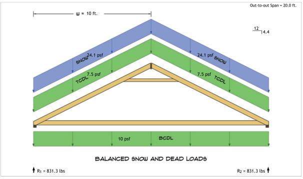
$R_1 = D + S = 349.1 \text{ lbs} + 482.2 \text{ lbs}$  $R_2 = D + S = 349.1 \text{ lbs} + 482.2 \text{ lbs}$
