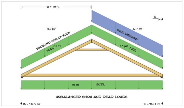
$R_1 = D + S = 349.1 \text{ lbs} + 188.4 \text{ lbs}$  $R_2 = D + S = 349.1 \text{ lbs} + 565.2 \text{ lbs}$
