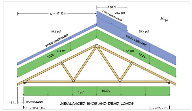
$R_1 = D + S = 2302.7 \text{ lbs} + 2762.1 \text{ lbs}$  $R_2 = D + S = 2302.7 \text{ lbs} + 4962.8 \text{ lbs}$
