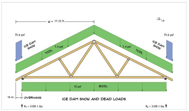
$$\begin{split} R_1 &= D + S = 2302.7 \text{ lbs} + 806.4 \text{ lbs} \\ R_2 &= D + S = 2302.7 \text{ lbs} + 806.4 \text{ lbs} \end{split}$$
