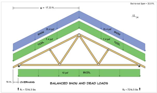
$$\begin{split} R_1 &= D + S = 2302.7 \text{ lbs} + 4913.8 \text{ lbs} \\ R_2 &= D + S = 2302.7 \text{ lbs} + 4913.8 \text{ lbs} \end{split}$$
