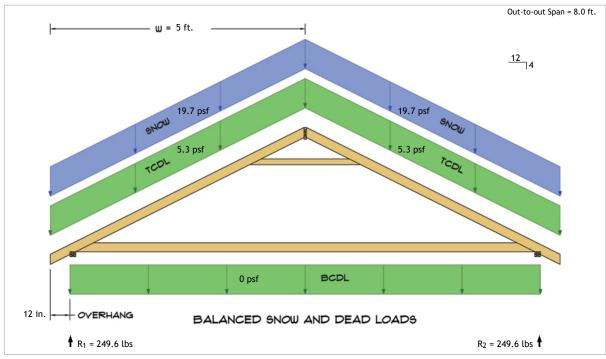
$R_1 = D + S = 52.7 \text{ lbs} + 196.9 \text{ lbs}$  $R_2 = D + S = 52.7 \text{ lbs} + 196.9 \text{ lbs}$
