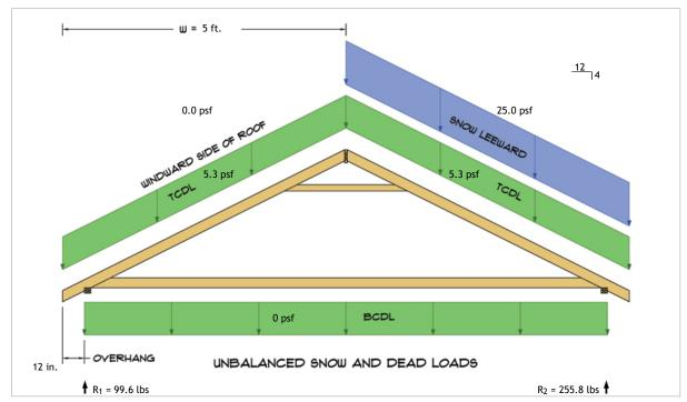
$R_1 = D + S = 52.7 \text{ lbs} + 46.9 \text{ lbs}$  $R_2 = D + S = 52.7 \text{ lbs} + 203.1 \text{ lbs}$
