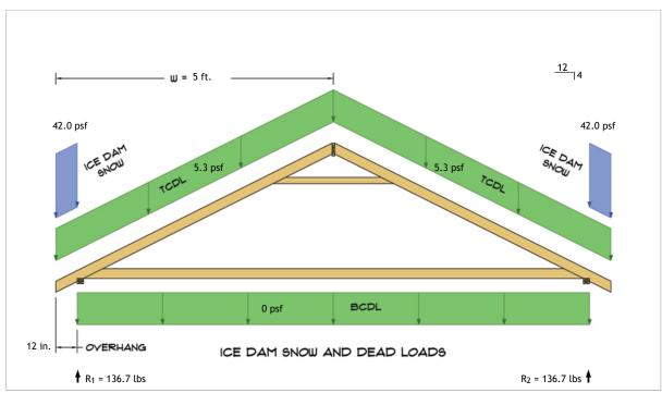
$R_1 = D + S = 52.7 \text{ lbs} + 84.0 \text{ lbs}$  $R_2 = D + S = 52.7 \text{ lbs} + 84.0 \text{ lbs}$
