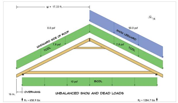
$R_1 = D + S = 394.1 \text{ lbs} + 264.8 \text{ lbs}$  $R_2 = D + S = 394.1 \text{ lbs} + 890.6 \text{ lbs}$
