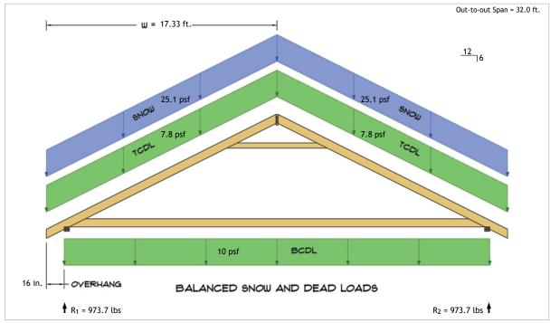
$R_1 = D + S = 394.1 \text{ lbs} + 579.5 \text{ lbs}$  $R_2 = D + S = 394.1 \text{ lbs} + 579.5 \text{ lbs}$
