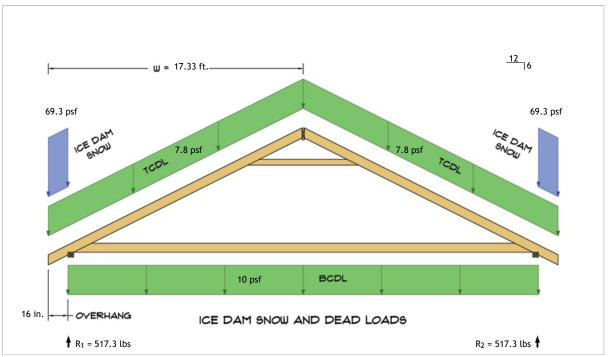
$R_1 = D + S = 394.1 \text{ lbs} + 123.2 \text{ lbs}$  $R_2 = D + S = 394.1 \text{ lbs} + 123.2 \text{ lbs}$
